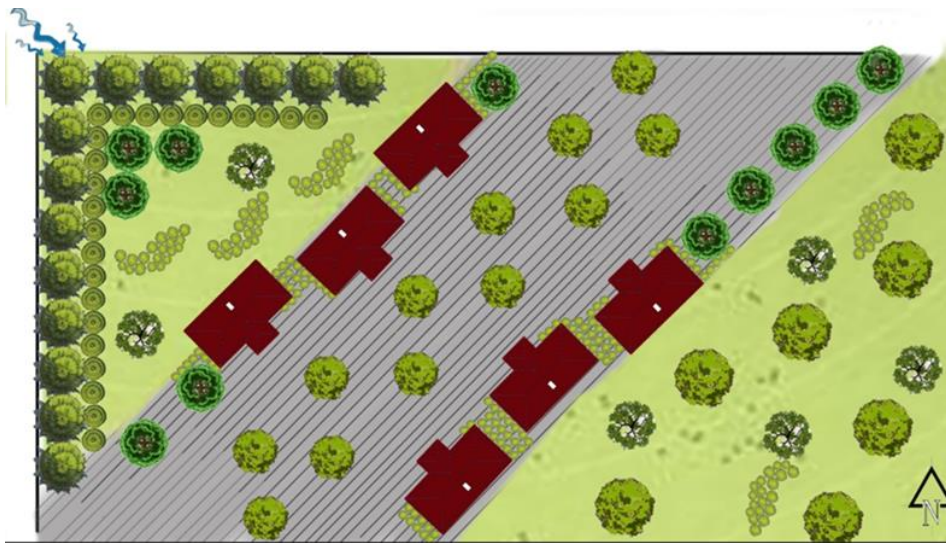
Figure 4. A design example that increases the thermal comfort level for the winter season of D type climate zones
