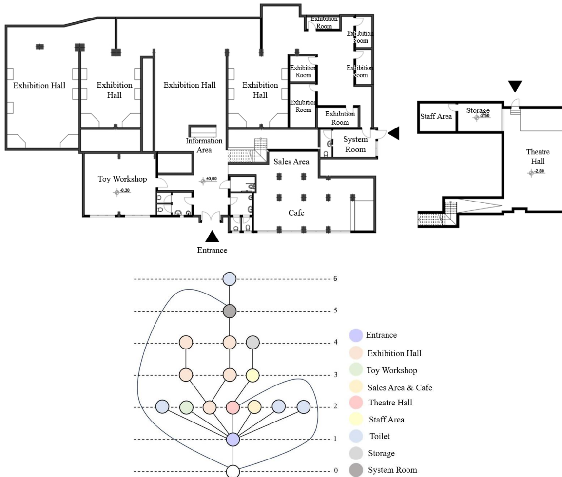
Figure 12. Canik Toy Museum entrance and basement floor plans (top), access graphic (bottom)
