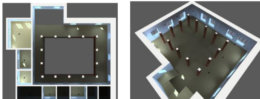
Figure 19-20. Hasan Sezai ground floor and gallery floor plan natural light modeling
