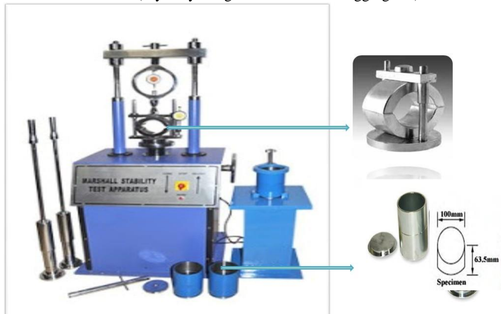
Figure 1. Marshall Stability Test
