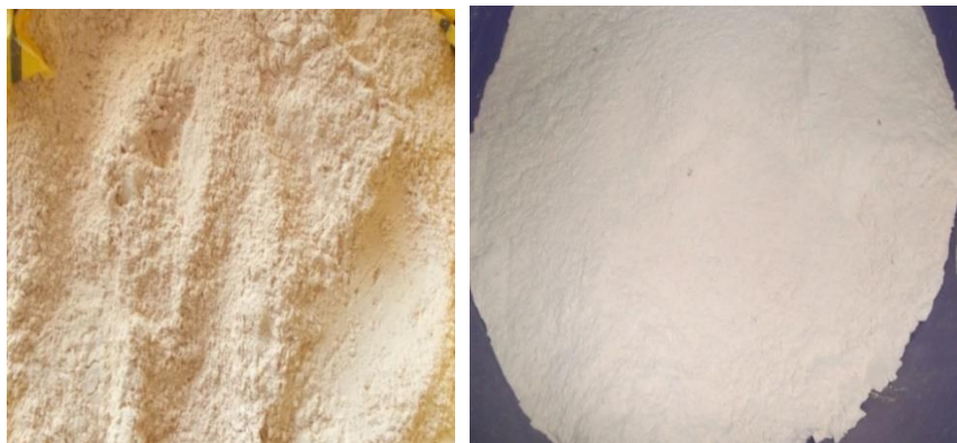
Figure 3a. A Sample of Oven Dried Kankara Clay. Figure 3b: A Sample of a Sieved Kankara Clay
