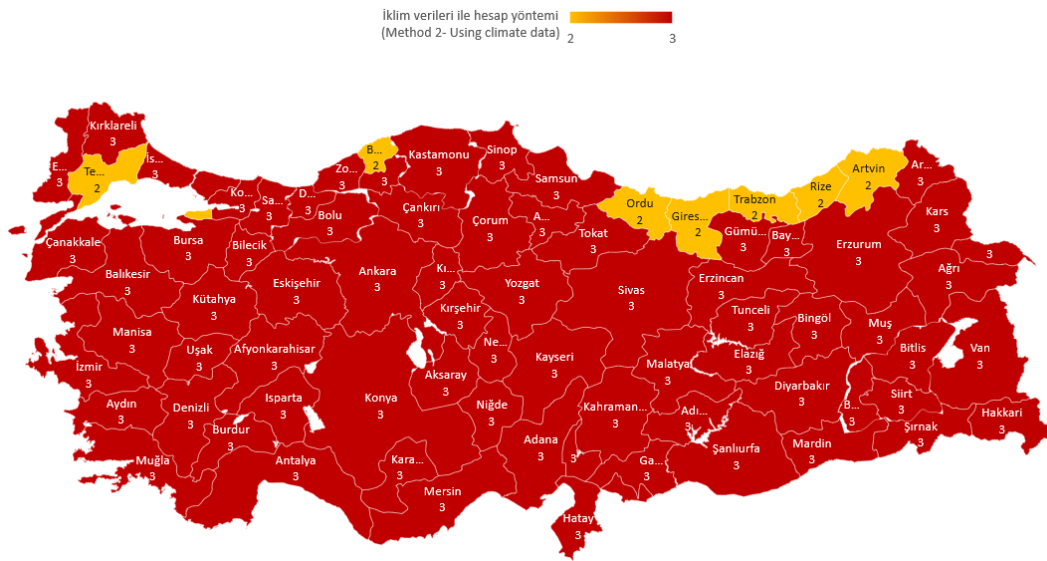
Figure 4. The “daylight provision performance” of the room according to the 2nd calculation method In all provinces of Turkey except Tekirdağ, between the two methods, there are differences in the “daylight provision performance” of the room. There is two level difference in Ardahan, Iğdır, Elazığ, and one level difference in other provinces (Figure 5).
