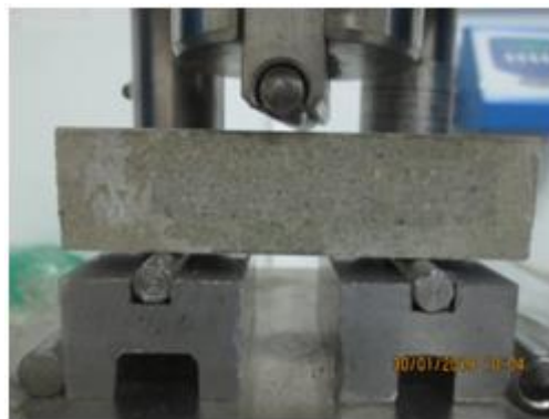
Figure 4. The principle of bending resistance on activated slag mortar
