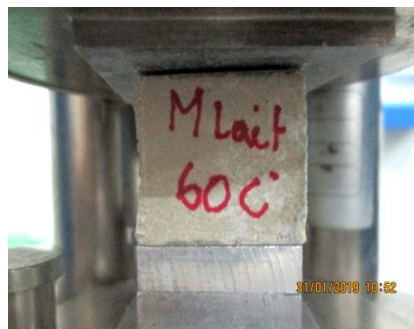
Figure 2. The shapes samples of alkalis activated mortars.
