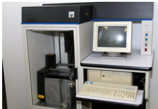
Figure 1. The first stereolithography 3D printer named SLA-1
