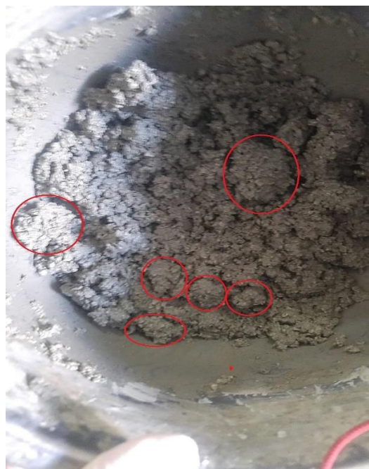
Figure 5. View of paper fibers causing agglomeration in cement-based mortars
