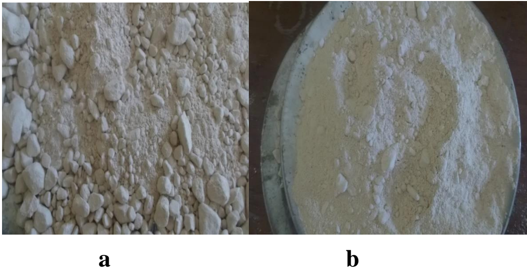
Figure 2a. A Sample of Raw Kankara Clay. Figure 2b. Sample of Beneficiated Kankara Clay
