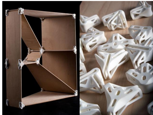
Figure 4. Joining detail produced with a 3D printer (Url-4)
