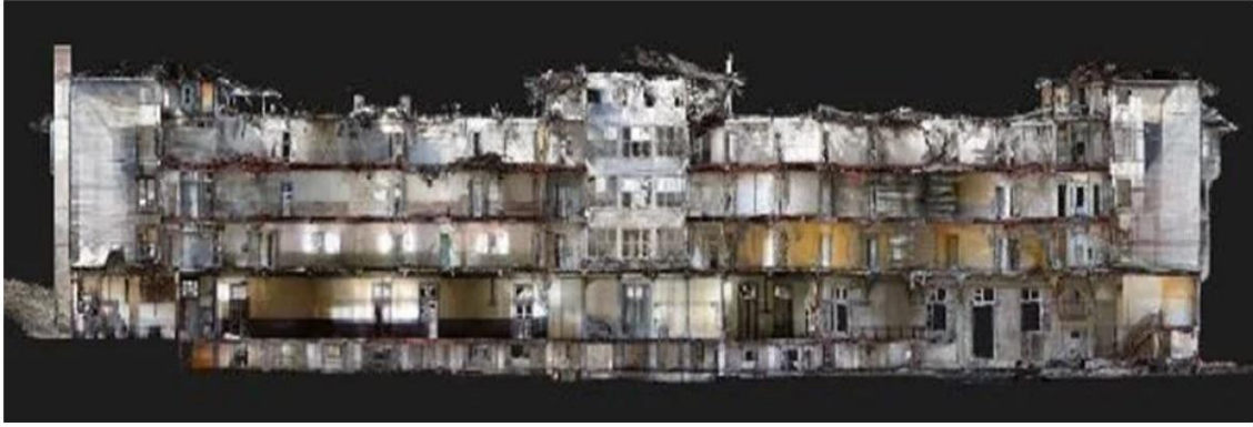
Figure 8. The survey study section of the Büyükada Greek Orphanage (Bimtaş, 2021)
