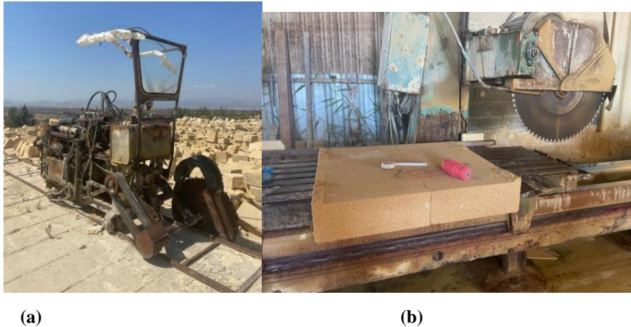
Figure 10. a. Dry stone cutting machine (Serhatköy Quarry) (Öge, 2022), b. Wet stone cutting machine (Alayköy Quarry) (Öge, 2022).
